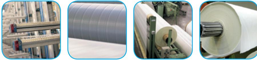
“Veranneman Technical Textiles is specialized in the production of impregnated open structure scrims. The open weave fabric is dip coated before being wound directly on the weaving loop (online coating). Main applications: reinforcement for PVC roofing and swimming pool membranes, non-woven filtration, construction, wind break nets and sign. Samples are available in 4 catalogues (sample books).
